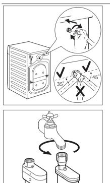
• Connect the hose to the appliance. Turn the inlet hose only left or right. Loose the ring nut to set it in the correct position.
